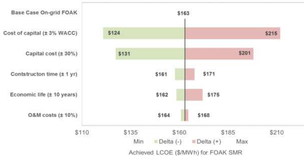
Figure 5: Tornado diagram illustrating cost drivers of SMRS. The figure shows the base case LCOE of $163 for an on-grid FOAK SMR. As shown, by applying different sensitivities to the base case you can see the impact resulting in min and max LCOEs. The sensitivities analyzed include cost of capital, capital costs, construction time, economic life and O&M costs.
