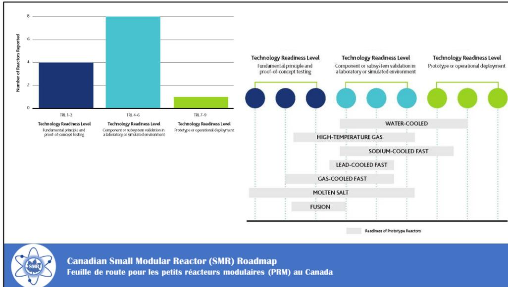
Generally, larger sized designs are closer to being commercially ready, and designs with less traditional or more unusual coolants (e.g. molten salt, gas) are further from being commercially ready. Each design will require development steps before a prototype or demonstration project can be launched. These steps will involve some work in Canada, and also work underway or planned in other countries.
